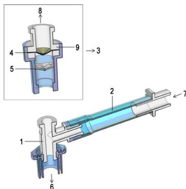
**Figure 1:** Components of sealing-type three-cavities ventilation
