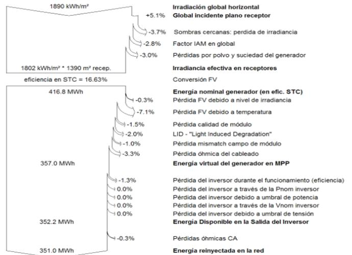
Figure 6: Loss and energy diagram of the photovoltaic installation
