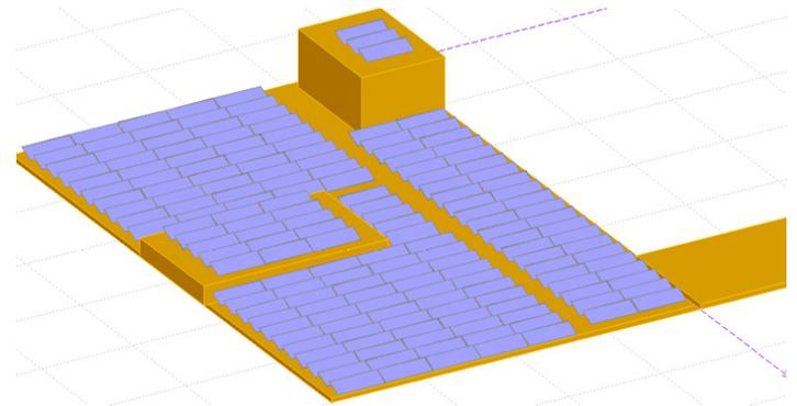
**Figure 3:** Disposition of the panels in the area.
