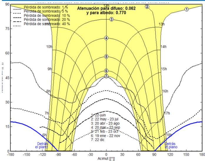
Figure 4: Installation shadow factor
