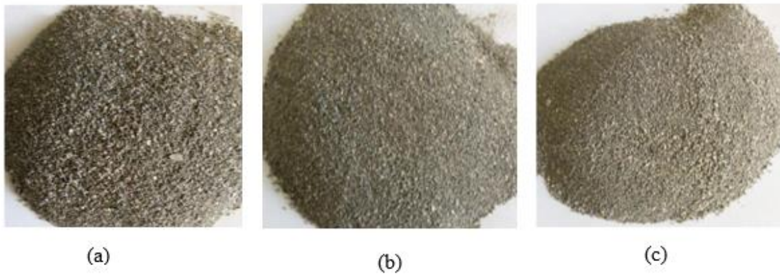
Figure 1: Granular Cement Particle Retained in Sieve Numbers 200 (a), 300 (b) and 600 (c)
