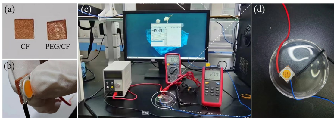
Figure 3: PEG/CF composite and copper foam (A), PEG/CF composite stuck to LED chip (B), thermal regulation performance evaluation system (C), zoom-in image of connected LED chip (D).
