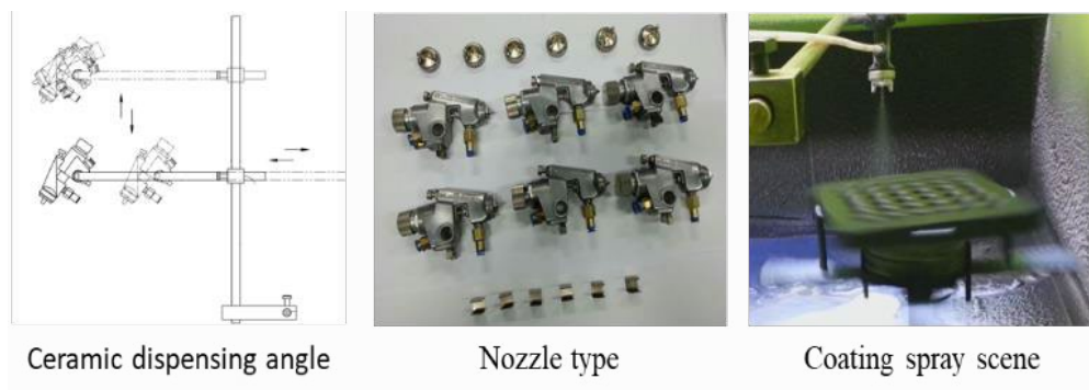
Figure 5: Automated Coating Dispensing System
