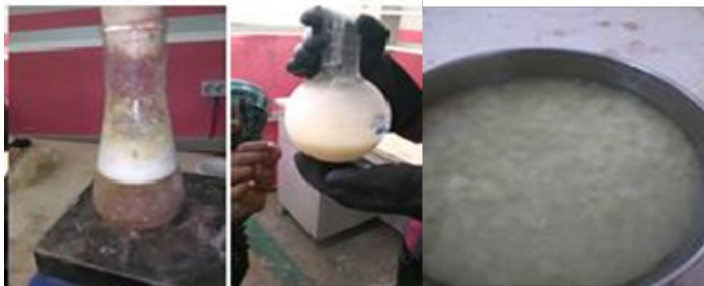
Figure 4: A photo showing Pulp bleaching, bleached pulp, and filtrated bleached pulp
