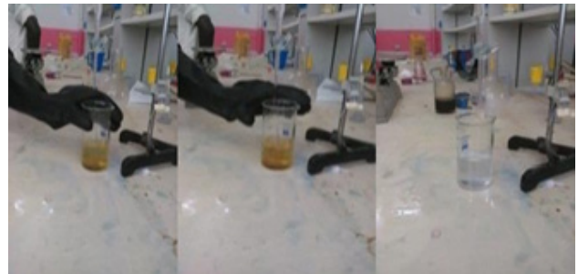
Figure 5: A photo showing Kappa number determination by titration
