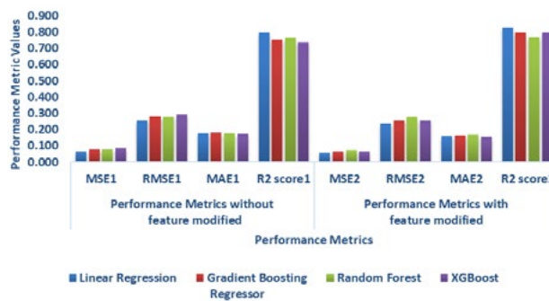
Figure 17: Mean Squared Error (MSE), Root Mean Squared Error (RMSE), Mean Absolute Error (MAE) and R-squared (R2 score) for linear regression, gradient boosting regressor, random forest, and XGBoost models
