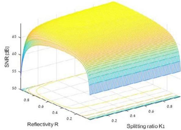
**Figure 8a:** OCT balanced system four beam splitter and Attenuator SNR (dB) as a function of splitting ratio  $K_1$  and mirror reflectivity R for  $\Gamma_s = 0.0001; \Gamma_x = 0.01$
