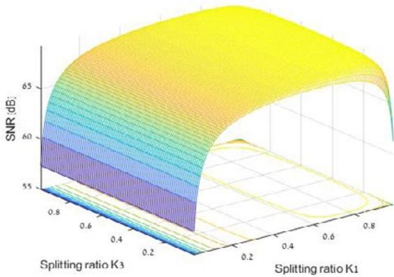
**Figure 8c:** OCT balanced system four beam splitter and Attenuator SNR (dB) as a function of splitting ratio  $K_1$  and  $K_3$  for  $\Gamma_s = 0.0001$ ;  $\Gamma_x = 0.01$
