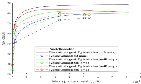
**Figure 6a:** OCT balanced system four beam splitter and attenuator SNR as a function of dc I for unpolarized light source ( $\nu = 0$ )
