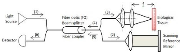
**Figure 1:** OCT Basic System Diagram
