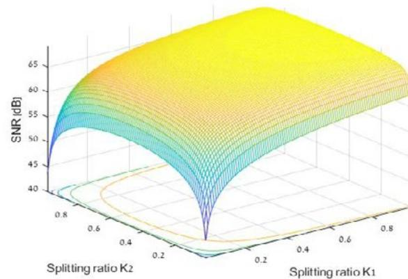
**Figure 8b:** OCT balanced system four beam splitter and Attenuator SNR (dB) as a function of splitting ratio  $K_1$  and  $K_2$  mirror reflectivity R for  $\Gamma_s = 0.0001; \Gamma_x = 0.01$
