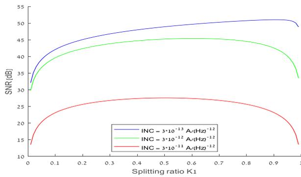
**Figure 7c:** OCT balanced system four beam splitter and Attenuator SNR (dB) as a function of splitting ratio  $K_1$  for  $\Gamma_s = 1 \times 10^{-6}, \Gamma_x = 1 \times 10^{-3}$
