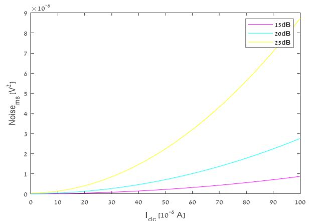
**Figure 5d:** OCT balanced system four beam splitter and attenuator noise as a function of  $I_{dc}$  (polarized), amplification 15dB, 20dB, and 25dB
