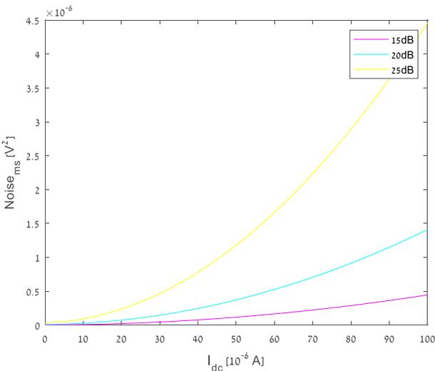
**Figure 5b:** OCT balanced system four beam splitter and attenuator Noise vs  $I_{dc}$  (unpolarized), amplification 15dB, 20dB, and 25dB
