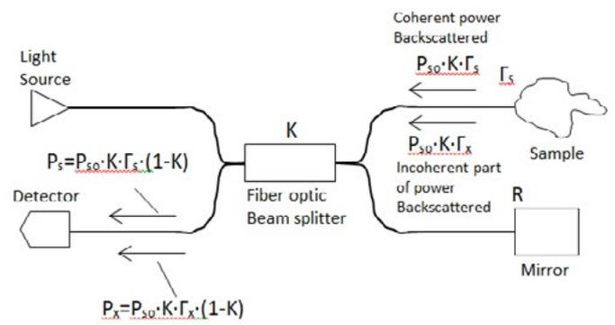
**Figure 2b:** Back Power Light from the Sample Tissue after Reflection and Back To the Detector
