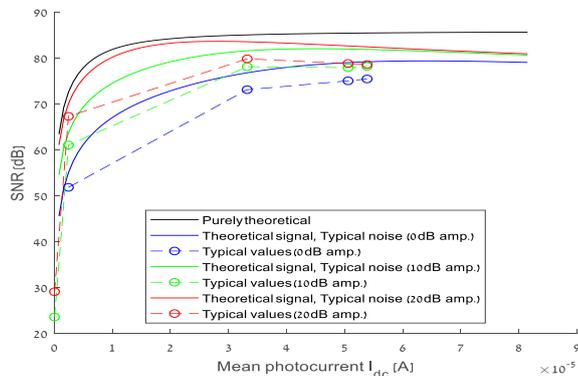
**Figure 6b:** OCT balanced system four beam splitter and attenuator SNR as a function of  $I_{dc}$  for a polarized light source ( $\nu = 1$ )
