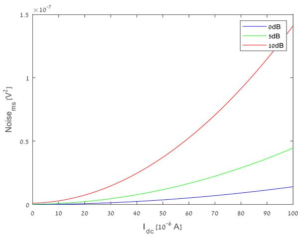
**Figure 5a:** OCT balanced system four beam splitter and attenuator noise as a function of  $I_{dc}$  (unpolarized), amplification 0dB, 5dB, and 10dB
