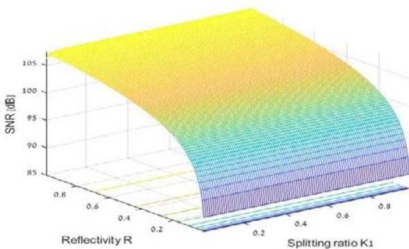
**Figure 8d:** OCT balanced system four beam splitter and Attenuator SNR (dB) as a function of splitting ratio  $K_1$  and mirror reflectivity  $R$  for  $\Gamma_s = 0.01$ ;  $\Gamma_x = 0.0001$
