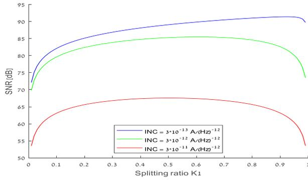
**Figure 7b:** OCT balanced system four beam splitter and Attenuator SNR (dB) as a function of splitting ratio  $K_1$  for  $\Gamma_s = 0.01, \Gamma_x = 1 \times 10^{-6}$
