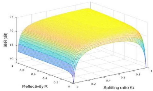
**Figure 8e:** OCT balanced system four beam splitter and Attenuator SNR (dB) as a function of splitting ratio  $K_1$  and mirror reflectivity  $R$  for  $\Gamma_s = 0.0001$ ;  $\Gamma_x = 0.01$  ( $R$ ) and coupling ratios ( $K_1$ ,  $K_2$ ,  $K_3$ , and  $K_4$ ) shows optimum SNR value for specific parameters values.
