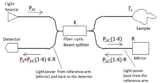
**Figure 2c:** Back Power Light from the Reference Arm (Mirror) Split by FO and Detect By the Detector
