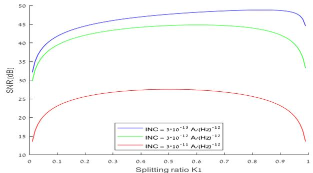
**Figure 7a:** OCT balanced system four beam splitter and Attenuator SNR (dB) as a function of splitting ratio  $K_1$  for  $\Gamma_s = 1 \times 10^{-6}$ ,  $\Gamma_x = 0.01$ .
