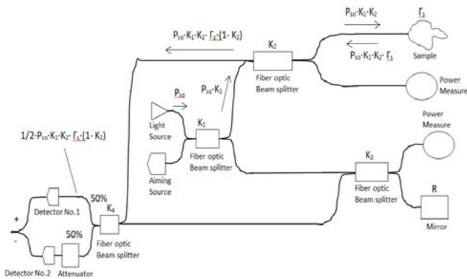
**Figure 4a:** Ongoing and back power light from the sample tissue after reflection, detects by the detector No.1 (coherent part), OCT balanced system with four beam splitters and attenuator.
