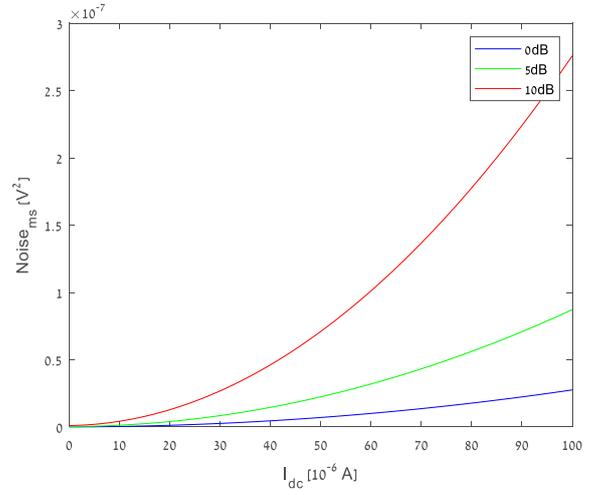
**Figure 5c:** OCT balanced system four beam splitter and attenuator noise as a function of  $I_{dc}$  (polarized), amplification 0dB, 5dB, and 10dB
