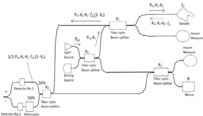
**Figure 4b:** Ongoing and back power light from the sample tissue after reflection, detects by the detector No.1 (incoherent part), OCT balanced system with four beam splitters and attenuator.
