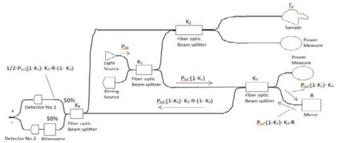
**Figure 4c:** Back power light from the reference arm (mirror) pass two beam splitters and detect by the detector, OCT balanced system with four beam splitters and attenuator.
