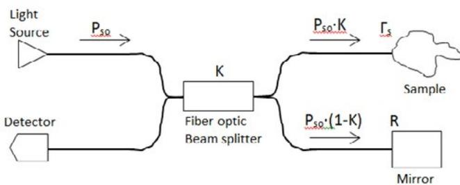
**Figure 2a:** Ongoing Power in Oct System after Fiber Optic Beam Splitter (Unbalanced System)
