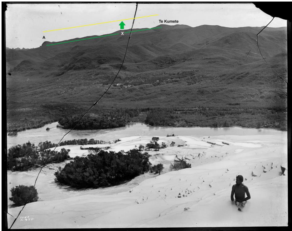
Figure 10. Crawford photograph with intervisible peaks from Hochstetter's survey on Kumete Ridge. The Skyline Gauge scale A to Te Kumete is in yellow and peak X the indicator is marked on the green scale (Tairāwhiti Museum).
