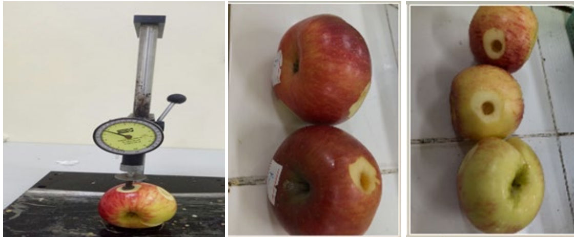
Figure 2: Measuring Firmness of Apple Fruit
