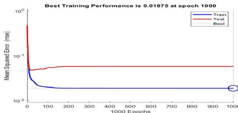
Figure 4: Network Performance for Traffic Characteristic Created with Simulation Data Using Bayesian-Regularization Algorithm
