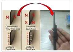
Figure 5: Magnetic Strips Polarities
