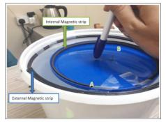
Figure 7: Magnetic strips arrangements in second experiment
