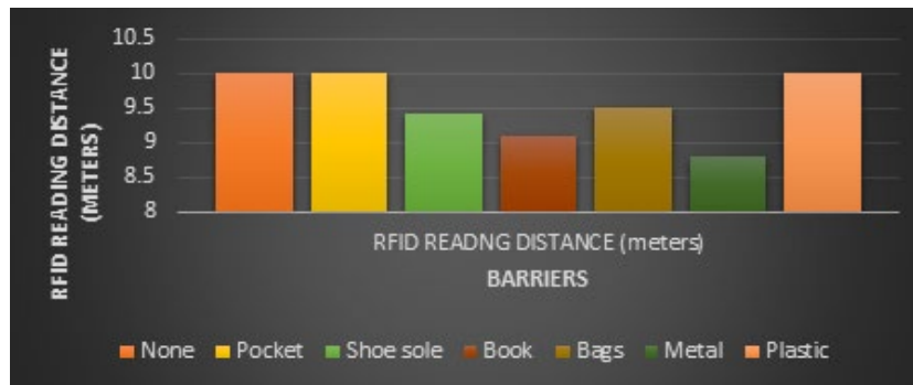
Figure: 2.4: Graph of RFID Reading Distance vs Barrier Type
