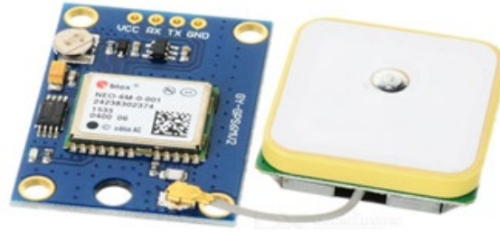
Figure: 2.1(c): ESP 32 SIM800L GPRS Module and NEO6m GPS Module
