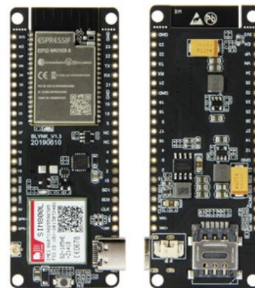
Figure: 2.1(a): ESP32 SIM800L Module (front-side) Figure 2.1(b): ESP32 SIM800L Module (back side)
