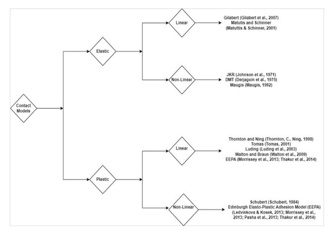
Figure 2: First Step for Selecting Contact Models
