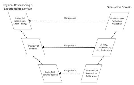
Figure 4: V-Model for Calibration and Validation (For e.g. Powders)
