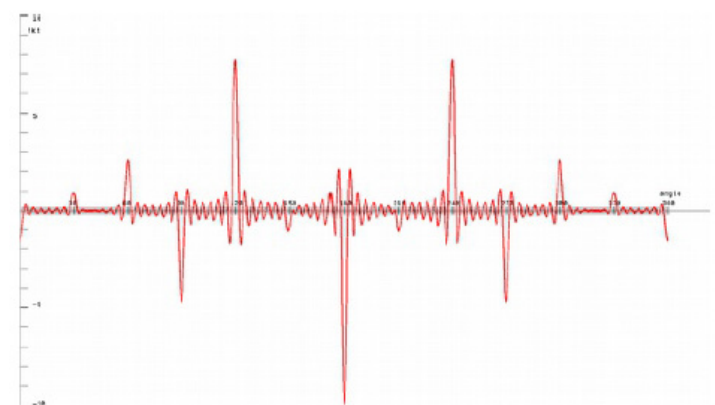
Figure 5: Correlation function H_{i,j} order according 7.to equation (10) with N=7 . The higher orders of the correlation function are suitable for resonance problems.
