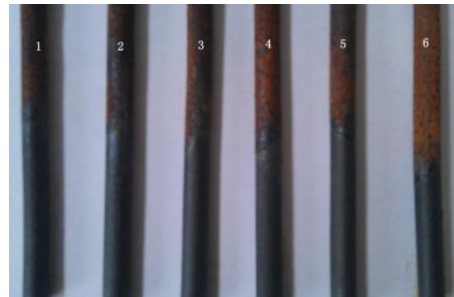
Figure 8: Effects of Various Pickling Solutions on Wire Rod Pickling At a Mass Concentration of 238 G/L Hydrochloric Acid
