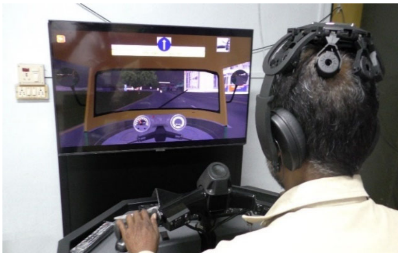
Figure 2: Photo of a Subject in the 3-Wheeler Driving Simulator with DSI-7 Wireless EEG Headset Mounted on Head
