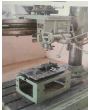
Figure 3: Fixture System in Drilling Machine
