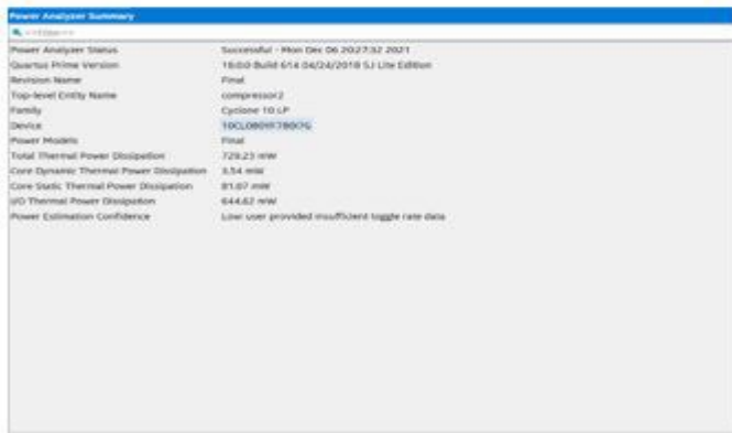
Figure 5: Power Analysis of the Existing 4:2 Compressor (Architecture 2)
