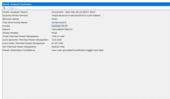
Figure 6: Power Analysis of the Proposed 4:2 Compressor
