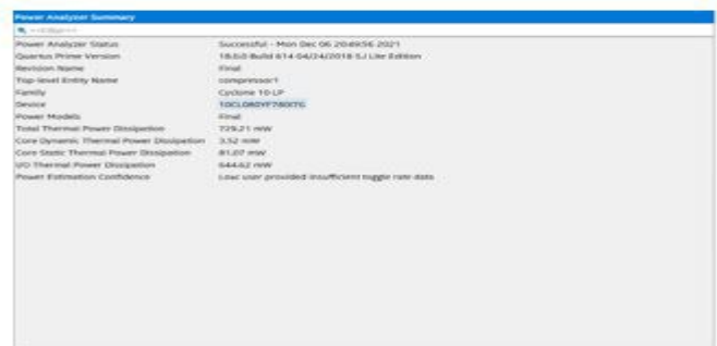
Figure 4: Power Analysis of the Existing 4:2 Compressor (Architecture 1)
