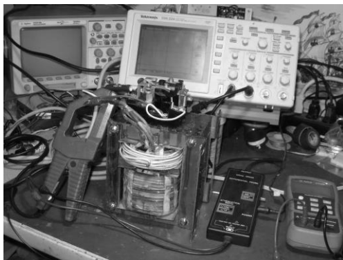
Figure 1B: Photograph of the 2 k.V.A test transformer M with tertiary winding P wrapped around the primary winding N!
