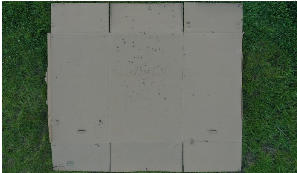
Figure 7: The Landing Platform From a Top View, after Completing The Measurements
