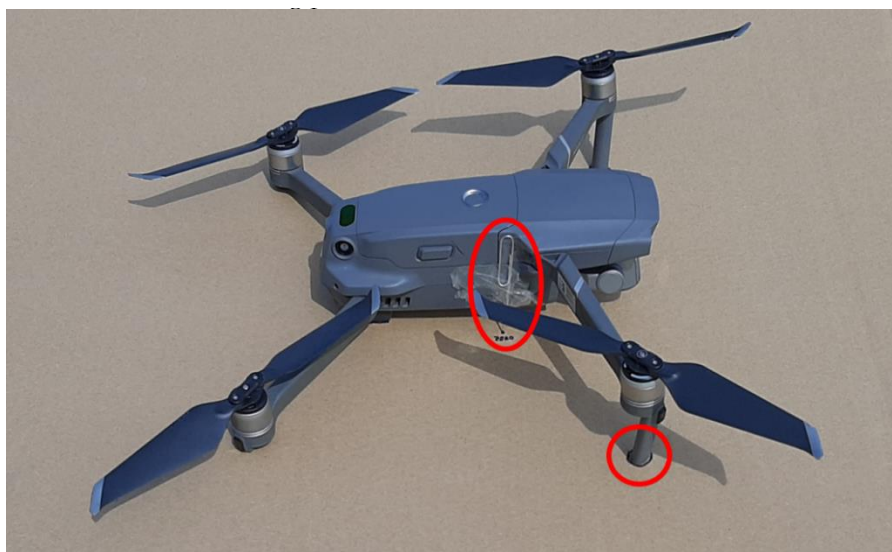
Figure 4: The DJI Mavic 2 Pro Used for the Measurements, with Necessary Markings on the Landing Platform and the Paperclip Marker Used to Indicate the Landing Points
