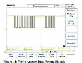
In Figure 11, we present a captured data frame representing the "Write Answer" within our data communication system. This figure showcases the response data frame generated in response to a "Write Request." As in the previous figures, the simultaneous presence of the request and response data frames is a result of the MAX485 chip's automatic transmission mechanism.
