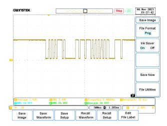
Figure 10: Write Request Data Frame Signals
