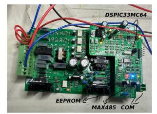
Figure 5: BETCOM Device Connected to Controlling System
