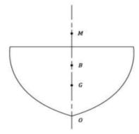
V is the volume of water displaced If the values of G & B are known GM can be determined. GM = BM+BG= BM+BO - OG
