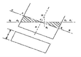
wV x BM $\theta$  = wb3L $\theta$ /12 BM = b3 L /12V = I/L Where I is the Second Moment of Area of the Water Plane Section
