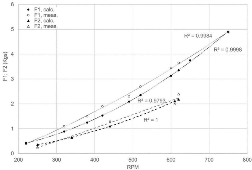
**Figure 5: Measured and Calculated F<sub>1</sub> and F<sub>2</sub> Peak Forces. (See also Figure 4)**
