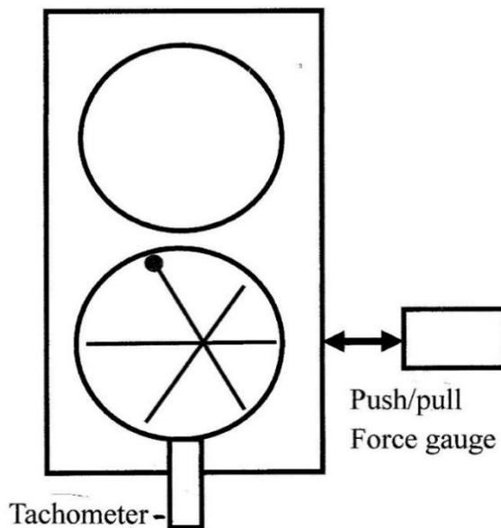
**Figure 4:  $F_1$  and  $F_2$  Measurements Set-Up**
