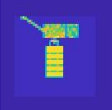
Figure 4: This illustrates how the Stochastic Search uses the nonnegative dynamic system to determine the noise-free image by the regular reduction of the Box size. We start with B_x = 80 and run n = 2 trials. Then we then select B_x = 60 and B_x = 40 , each having two trials. The satellite is 50% the size of the 40 pixel box. Consequently we discover that the final pair of images are fully correlated and thus are the noise-free image. The parameters of the dynamic system are \varepsilon = 10^{-6} and \beta = 0.7 . Each trail was computed for 3000 iterations in approximately 3.5 seconds using an Apexx W Class, thus producing the noise-free image in 21
