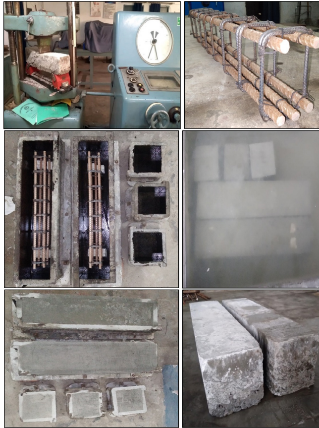
Figure 5: Experimental Setup of the Specimen & Casting of Beam
