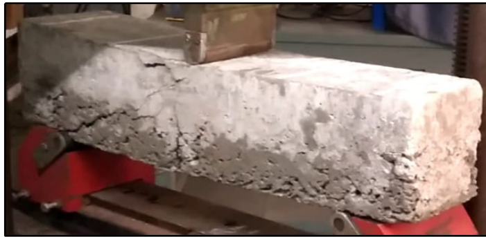
Figure 10: Beam-1 Fifth Stage Deflection at Load 34.33 kN
