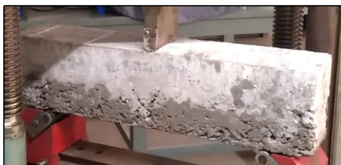
Figure 6: Beam-1 First Stage Deflection at Load 9.8 kN
