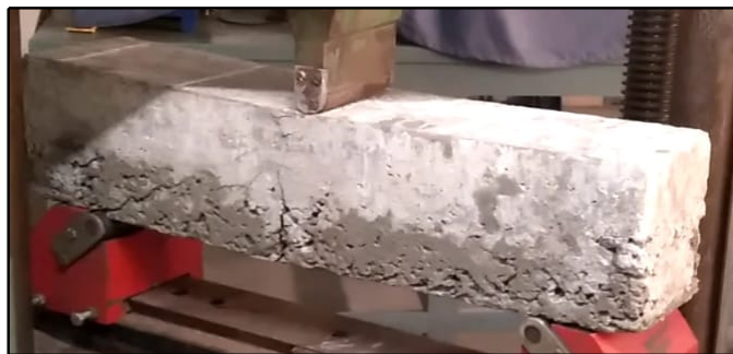
Figure 9: Beam-1 Fourth Stage Deflection at Load 29.42 kN
