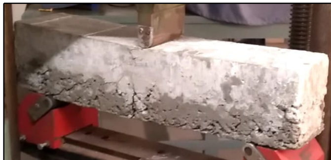
Figure 8: Beam-1 Third Stage Deflection at Load 24.52 kN
