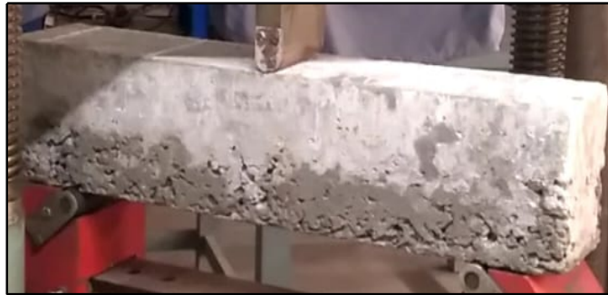
Figure 7: Beam-1 Second Stage Deflection at Load 19.2 kN
