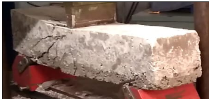
Figure 11: Beam-1 Sixth stage deflection at load 37.26 kN
